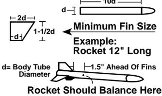
The third rule is to place the fins as far back on the rocket as possible. Generally, this means that the rear edge of the fin will meet the rear end of the body and the fin will be swept back. Do not place any fins ahead of the center of gravity!
