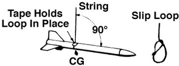
With the rocket suspended at its center of gravity, swing it overhead in a circular path. If the rocket is very stable, it will point forward into the wind created by its own motion. Some rockets which are stable will not point forward of their own
