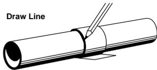
(2) Slide a stage coupler or expended engine casing into the tube – center it under the cut position to support the tube.
