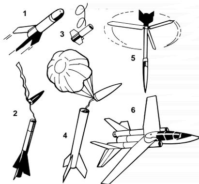
1. Featherweight Recovery, 2. Streamer Recovery, 3. Tumble Recovery, 4. Parachute Recovery, 5. Helicopter Recovery, 6. Glide Recovery.
