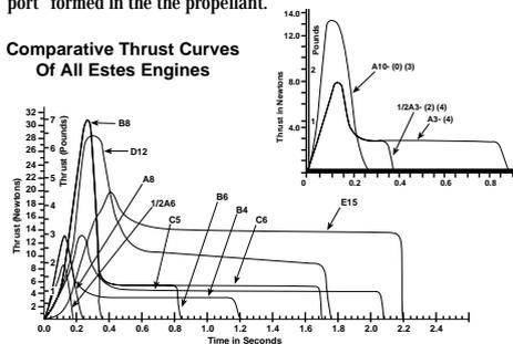
The most common model rocket engine is the end-burner, which has a shallow port. This design is used in many Estes engines and is especially effective with lightweight high performance rockets. The high initial thrust boosts the rocket to a suitable flying speed almost immediately; thrust then drops to a lower sustaining level to maintain speed and gain the most distance with the least fuel consumption.
