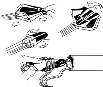
If the parachute has been packed in the model for an extended period, re-pack the 'chute just prior to launch. Dusting the parachute with talcum powder before packing will also increase the chances of a successful deployment. It is especially important to follow these precautions on cold days because the low temperature makes the plastic parachute material less flexible.
