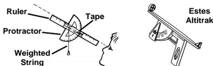
The distance from the launch area to the tracking station should be approximately equal to the altitude expected for an average rocket flight to be tracked. This distance is called the "baseline" and its length should be carefully measured. The tracker should have a clear view of the launch area and should not be looking into the sun.
