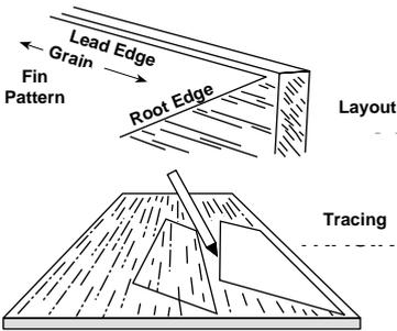
Use a metal straightedge whenever possible. Hold the knife blade at a 90° angle to surface being cut, and handle at about 45° for clean cut. If blade is dull or held too high, balsa tends to tear. A razor saw blade may be required to cut thicker balsa.
